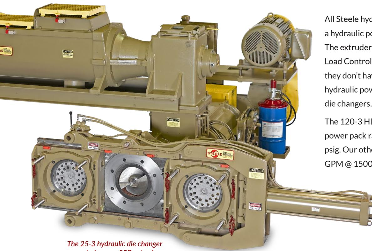
*The 25-3 hydraulic die changer mounted on our 25B extruder.*
