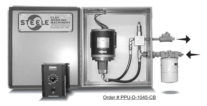
The V-1 Oil System, compared to other die lubrication pumps, is less expensive to purchase initially and requires fewer and less costly replacement parts. It will pump oil-based die lubricants and even used (clean) hydraulic fluids. Adjustments in volume are easy to make because the variable speed motor control may be located at the machine operator's control panel.
